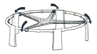
Spread out the net and attach it to the hooks in 4 places, making an "X" shape with the net, Note that the net goes over the rim and attaches to the hook underneath.
